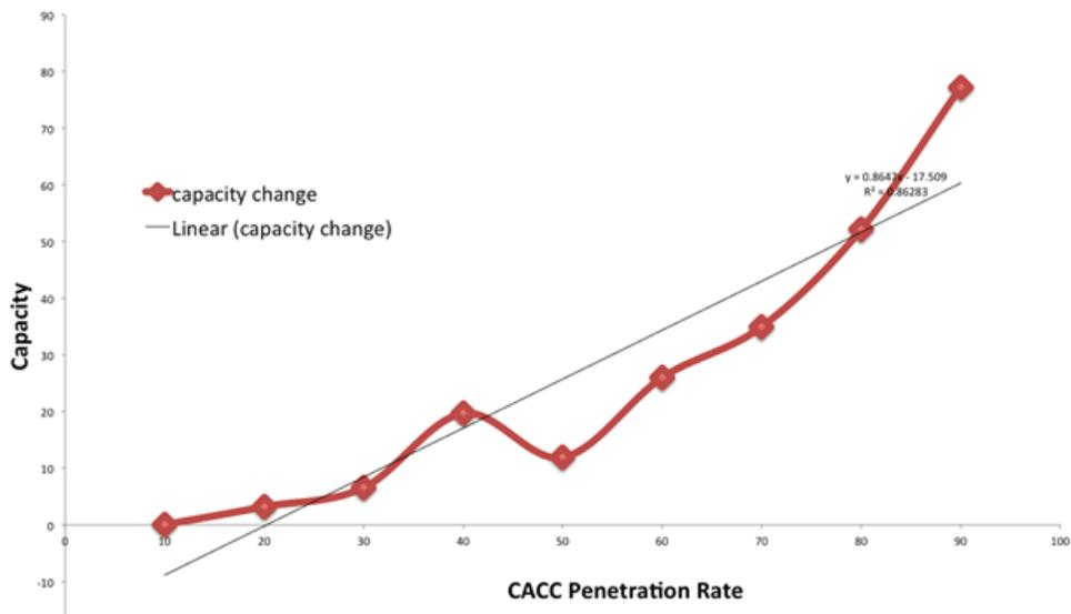
Fig. 1. Capacity change vs. market penetration of CACC
