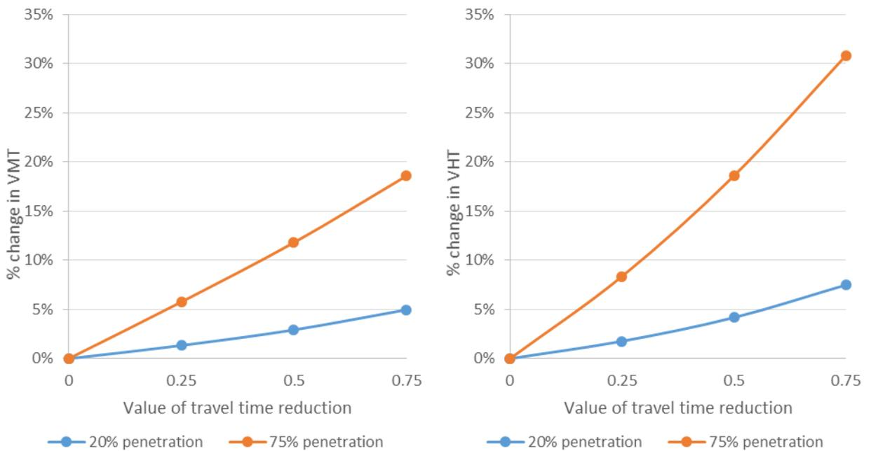
Fig. 3. (a) VMT change and (b) VHT change vs VOTT change by market penetration (no capacity change)
